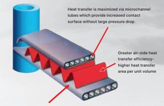
Brazed tube to fin joint where heat transfer is improved without air gaps.
