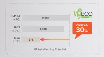
R32 is outstanding for their environment friendly properties as It does not contribute to ozone depletion and preserve global climate changes. The R32 refrigerant has zero Ozone Depletion Potential (ODP) and reduction of the global warming potential up to 30% when compared with R410A & R22.
