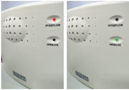
Operating LED Light (Green) and overflow LED light (Red)
